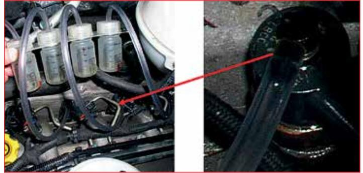
*Using small bottles and 8mm plastic tube to measure CRD leakback from injectors to return system.*
